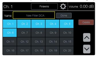
5. Enter a name for the new group using the onscreen keys. Press the onscreen Enter button when you are finished entering the name or use the onscreen Back button to leave the page without renaming the group.
