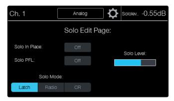
**Latch** is the default Solo mode. When Latch Solo mode is active, you can solo multiple channels and buses at once.
