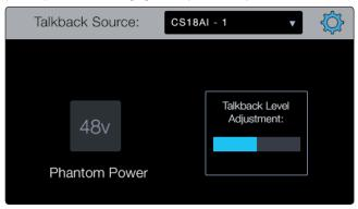
Power User Tip: While the talkback can be assigned and unassigned to multiple aux buses at once, each aux mix provides its own individual level control for the talkback via the Returns layer.
