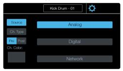
Name the channel by touching the name while on the Channel Settings screen. This will bring up the Text Entry screen. From here you can customize the name of the channel. The name will be displayed in the touchscreen when the channel is selected and in the scribble strip display for that channel. The name is also synchronized with all StudioLive UCNET devices and software, such as UC Surface, QMix-AI, and Capture, so you only have to name it once.
