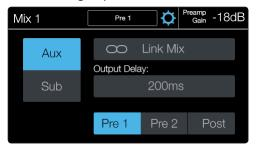
Name the mix by touching the name while on the Mix Settings screen. This will bring up the Text Entry screen. From here you can customize the name of the mix. The name will be displayed in the touchscreen when the channel is selected and in the scribble strip display for that channel. The name is also synchronized with all StudioLive UCNET devices and software, such as UC Surface, QMix-AI, and Capture, so you only have to name it once.
