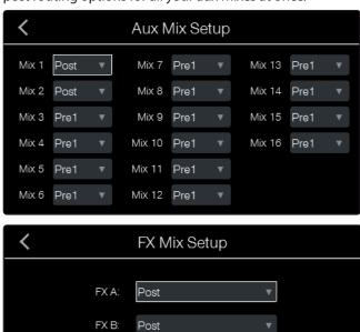
By default, all aux mixes are set to Pre 1. This places the send of every input channel to each aux bus before the fader, limiter, EQ, and compressor but after the Polarity Invert switch, highpass filter, and gate.
