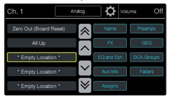
5. Press the Store button in the Master Control area. The text entry screen will appear, allowing you to name the scene. When you're done, press Enter to save the scene.
